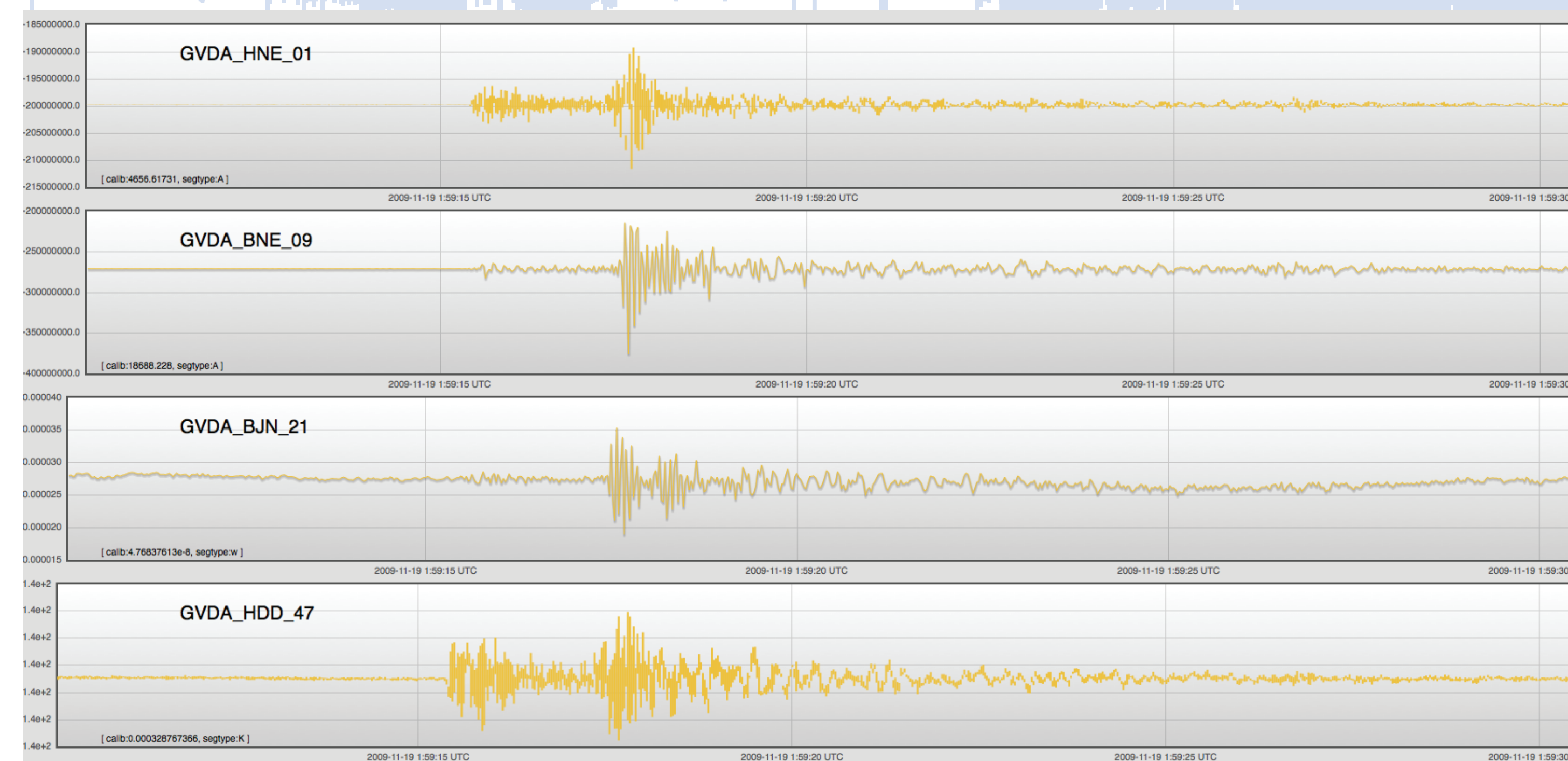
FIGURE 5. HIGH AND LOW DENSITY PLOTS Efficient rendering of high and low density traces. Channels BNE and BJN are 40 Hz channels returned as JSON object less than 25 KB containing 819 2-tuple elements in the format [time,value]. Channels HNE and HDD are 200 Hz channels returned as JSON objects of less than 33 KB containing 819 3-tuple elements in the format [time,max,v,min-v]. Data for plot provided by the Institute for Crustal Studies, University of California Santa Barbara, Santa Barbara, CA 93106-1100
