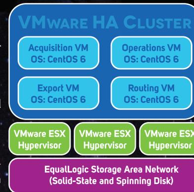
Block diagram showing the major components of the VMware stack. The VMware images and the large data volume are located on the shared SAN storage.
