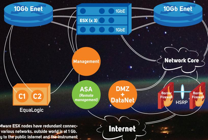
All three VMware ESX nodes have redundant connections to the various networks. outside world is at 1 Gb. Connectivity to the public internet and the instrument network is through the existing network core.
