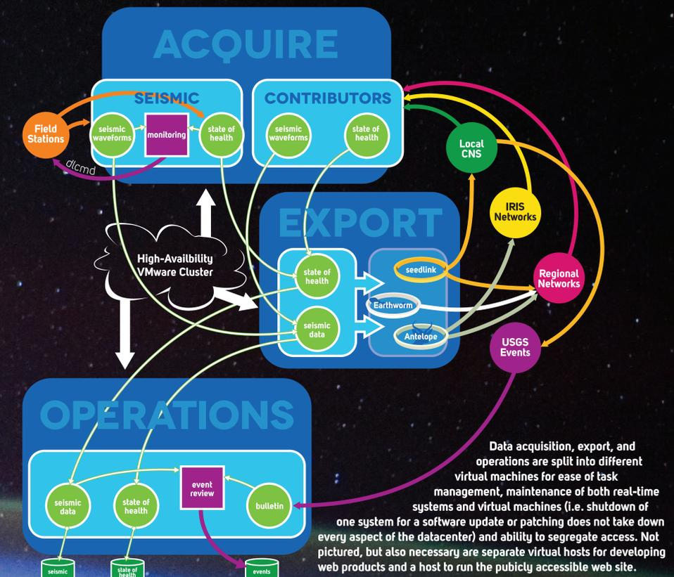
Data acquisition, export, and operations are split into different virtual machines for ease of task management, maintenance of both real-time systems and virtual machines (i.e. shutdown of one system for a software update or patching does not take down every aspect of the datacenter) and ability to segregate access. Not pictured, but also necessary are separate virtual hosts for developing web products and a host to run the publicly accessible web site.
